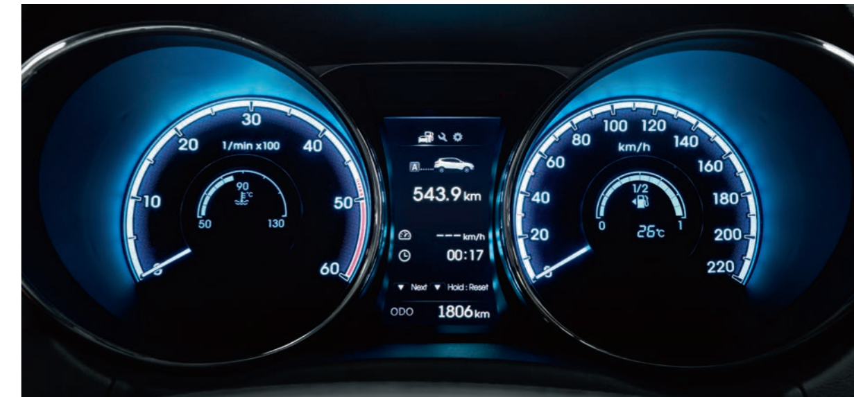
Information display. The new optional instrument cluster includes a 4.2" TFT-LCD menu-controlled screen, displaying information concerning vehicle operational status.
