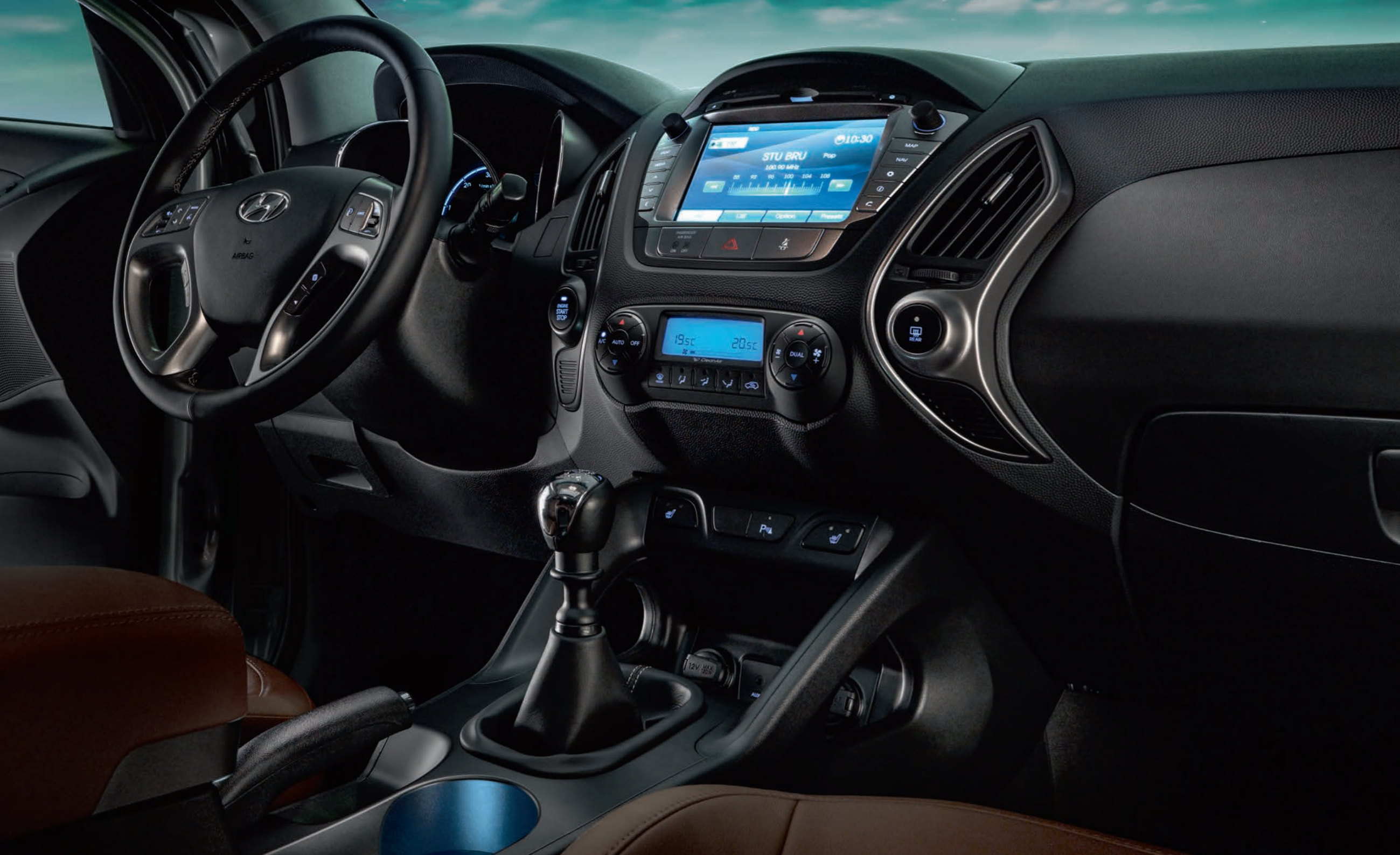
Information display. The new optional instrument cluster includes a 4.2" TFT-LCD menu-controlled screen, displaying information concerning vehicle operational status.
